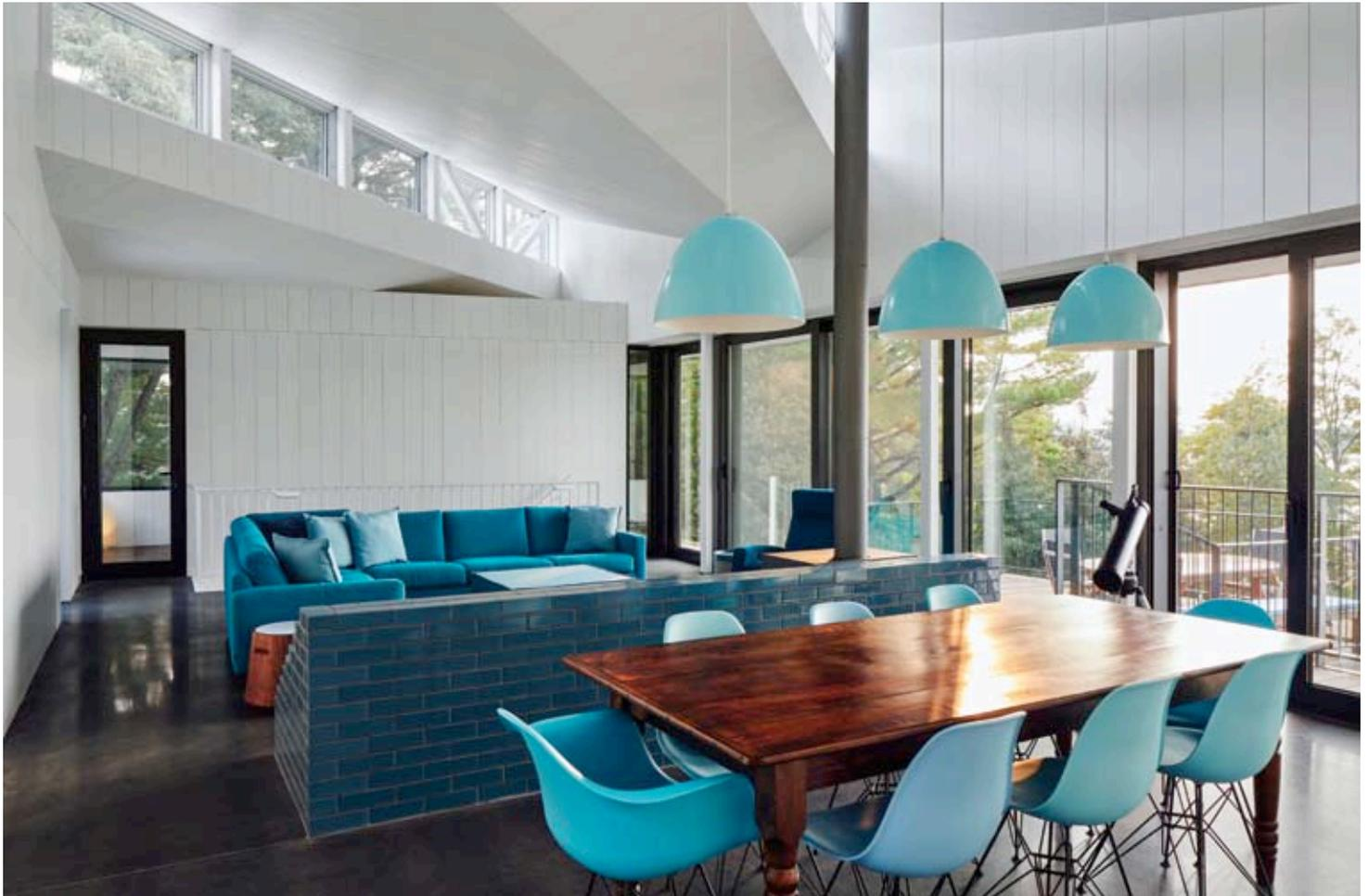
This distinctive feature allows for a series of vertical skylights to let in daylight while significantly avoiding heat gain.
