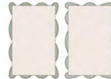
3. Green spaces for natural light and ventilation are added along the entire envelope of the building due to restricted plot size and density.
